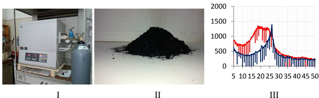
Figure 1. High temeperature vacuum furnace (I) for thermal reduction rGO to graphene (II); (III) XRD patterns of rGO and thermally reduced graphene oxide (rGO).
